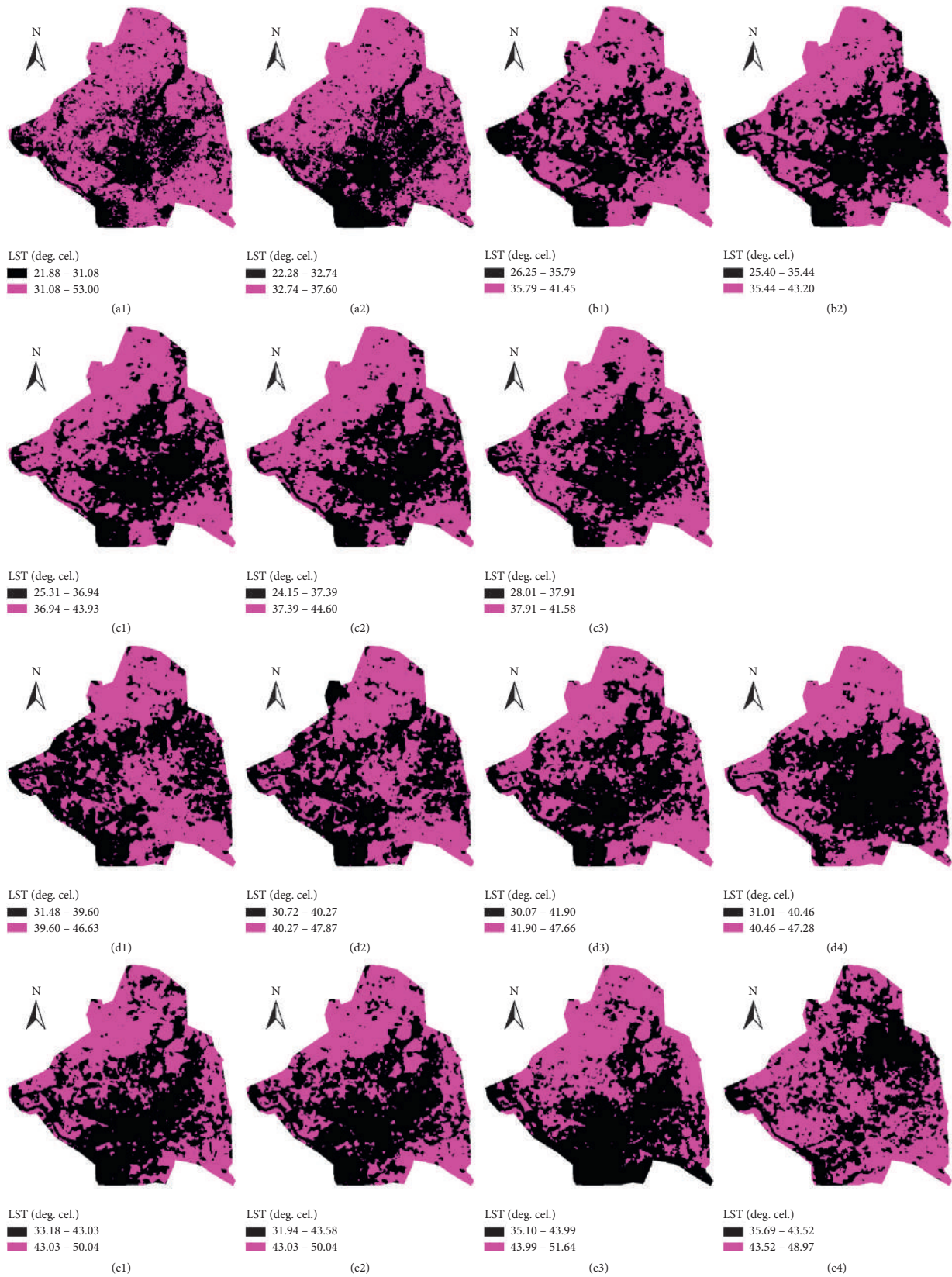
FIGURE 6: The area above mean LST (pink portion) and the area below mean LST (black portion): (a1-a2) 2002, (b1-b2) 2006, (c1-c3) 2010, (d1-d4) 2014, and (e1-e4) 2018.
